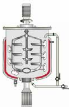
Single way mixing & external circulation
