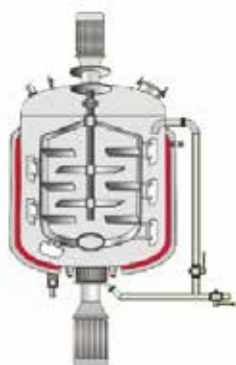
Single way mixing & external circulation
