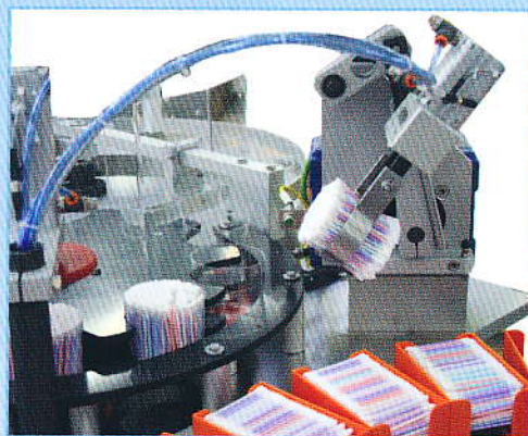
Pick-up robot with brushless motor detail
