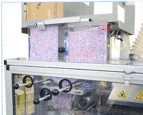
Sticks infeed double hopper. Up to 8 boxes storable
